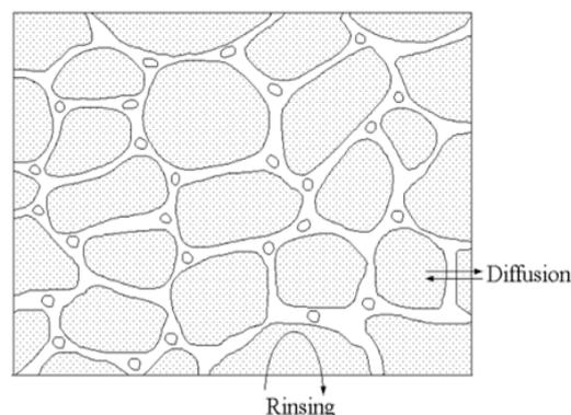
Figure 3: Schematic diagram of vegetal cell structures during the normal soaking extraction process with 2 different mechanisms involved: 1) Rinsing and 2) Difussion (Zubairi et al., 2016)
